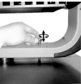
The second stop, located between the yoke and lamp housing, inhibits tilt
