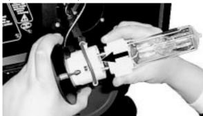
7) Replace the lamp assembly in its original position and refastern the 3 screws previously removed.
